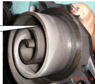
The bearing is seriously worn, and completely damaged
