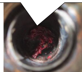
The filter is blocked by impurity; the compressor suction will be abnormal
