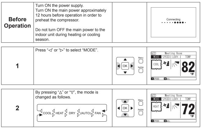
Automatic heating/cooling operation requires extra settings. Contact your distributor or contractor for details.
